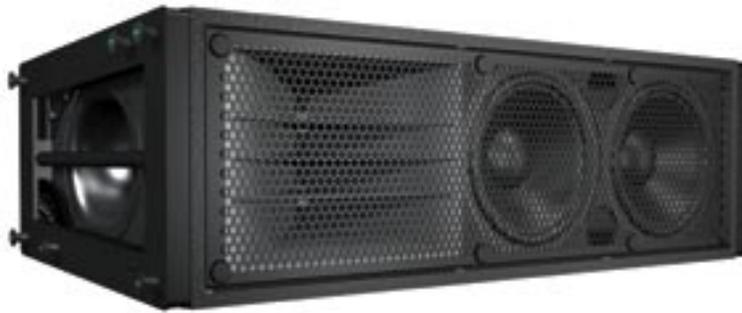
The M2D™ compact curvilinear array loudspeaker brings numerous advantages to mid-sized venues that require tight vertical pattern control with medium-to-long throw. Its operating frequency range is 60 Hz to 16 kHz, with maximum peak output of 136 dB SPL (each cabinet) at 1 meter.
